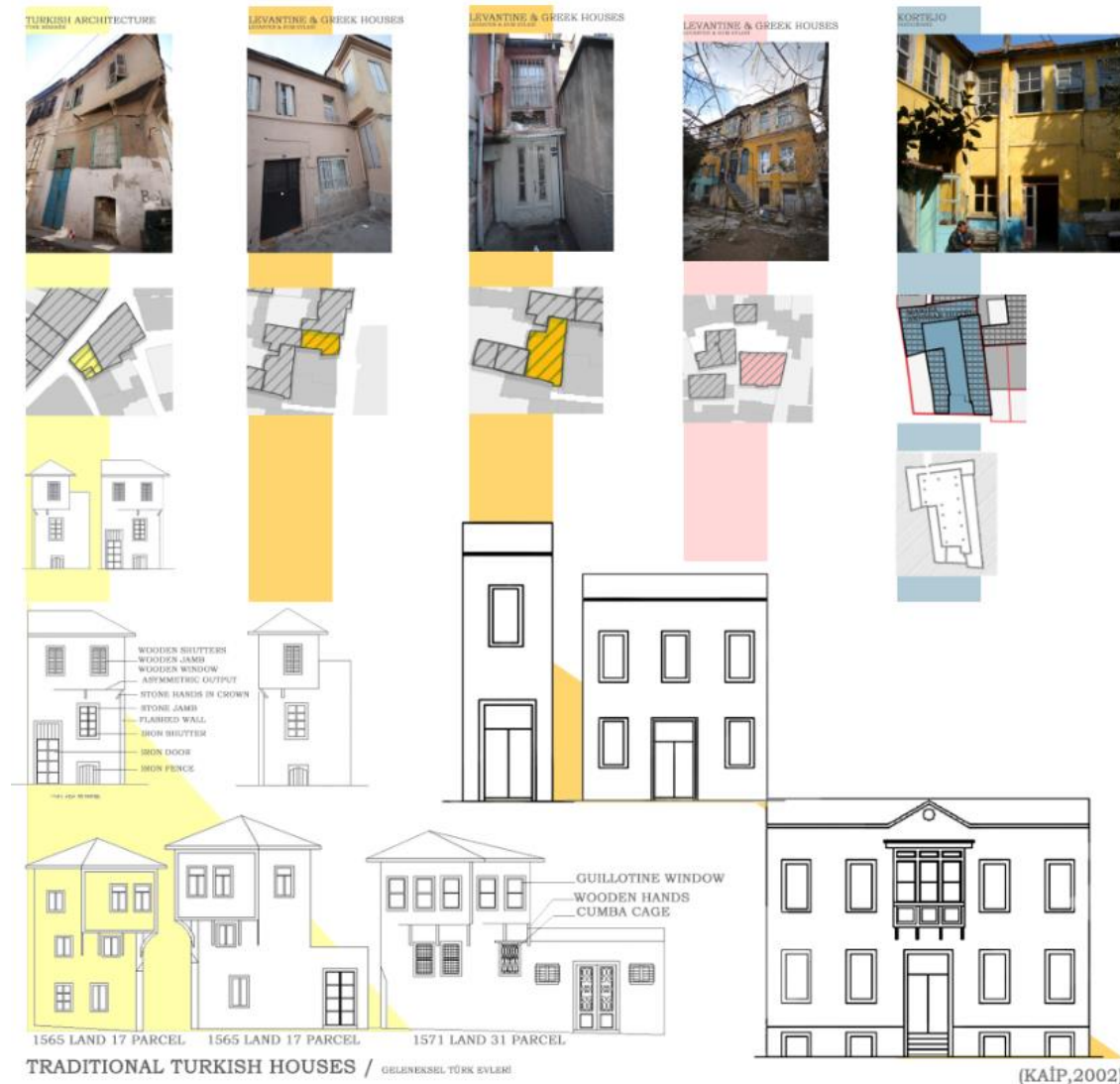
Figure 60: İzmir Traditional Housing Architecture
